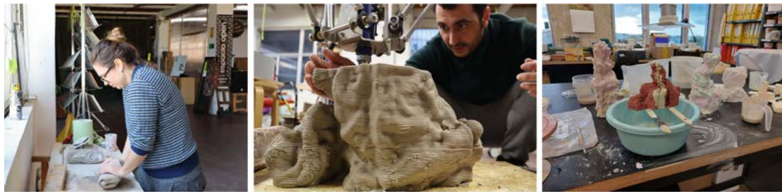
Fig. 7. Working with ceramics (from left to right): 1. mixing clay with water and filling a 3D printer tank with it. 2. supervising 3D printing process 3. glazing process.
